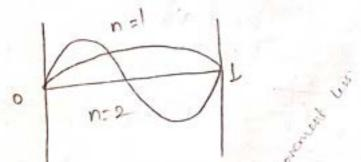
In this case, Stationary waves are set up with specific wavelength such that  $n\left(\frac{\lambda}{2}\right)=1$ .
